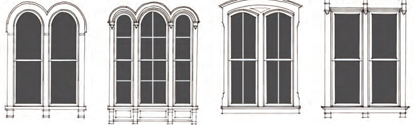
Paired windows are most often 1 over 1 or 2 over 2. Bracketed heads are more common on rectangular windows and pairings.
